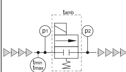
$$\begin{aligned} t_{\min} &= -45^{\circ}\text{C} \\ t_{\max} &= +125^{\circ}\text{C} \\ t_{\text{amb}} &= -40^{\circ}\text{C} \dots +80^{\circ}\text{C} \end{aligned}$$
